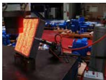
Preheating Burners before welding / assembly
