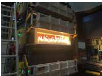
Flame Curtains for heat Treatment Furnaces
