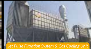
Jet Pulse Filtration System & Gas Cooling Unit
