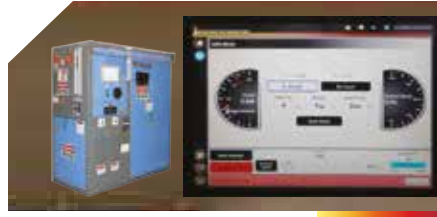
Computer controlled VIP induction melting power units
